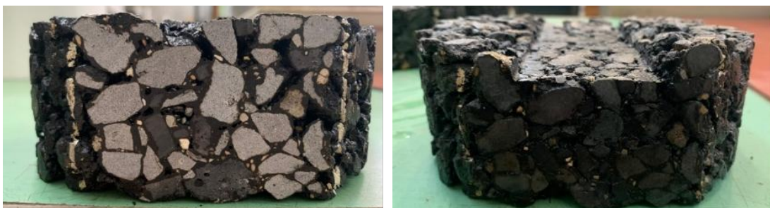
Figure 18 - Reorganisation of the aggregate structure and the reduction of voids in different Open-Graded asphalt mixtures
