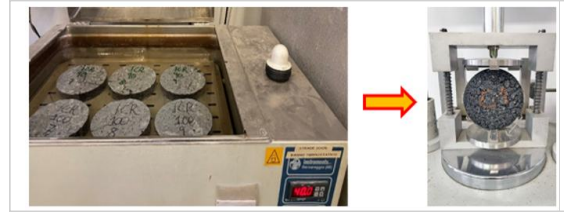
Figure 15 - ITS wet: samples conditioning 72h at 40°C, test temperature 25°C
