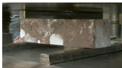
Figure 5 – Photo - 2005. Testing of samples of beams made from cutting out the lower layer of cinder concrete coating for bending strength (the structure of the beam is heterogeneous - the filler is a local gravel-sand mixture)
