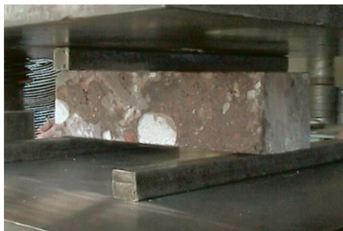
Figure 5. Photo - 2016. Testing of samples of beams made from cutting out the lower layer of cinder concrete coating for bending strength (the structure of the beam is heterogeneous - the filler is a local gravel-sand mixture)
