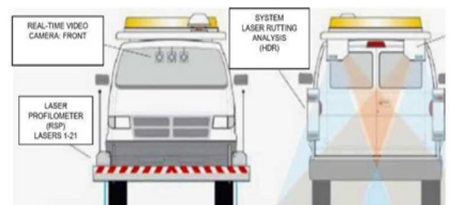
Fig. 2. Road monitoring and data collection system (front and rear views).
