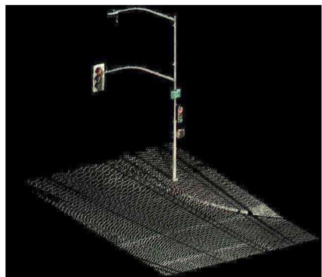
Fig. 6. Point cloud of a pole at a road intersection.
